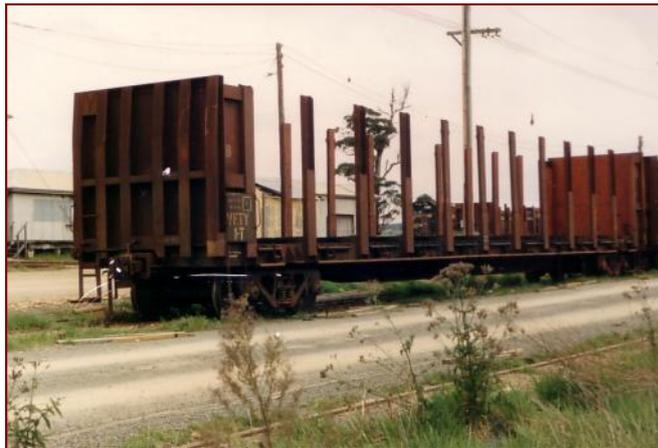
VFTY TIMBER WAGON - Thirty of these large wagons were built for the timber traffic between Orbost and Melbourne.
