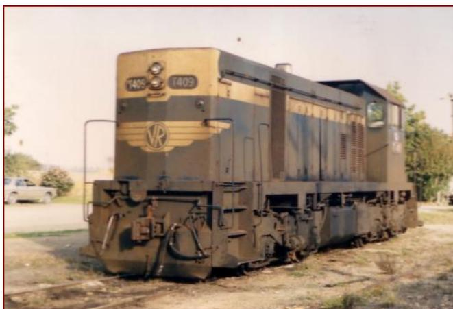
DEISEL ELECTRIC LOCOMOTIVE - This is a Series 3 'T' Class Locomotive often used in pairs to haul the timber trains out of Orbest.
