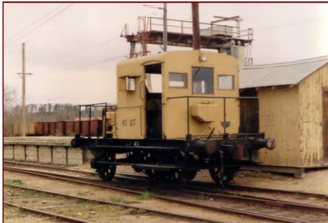
**RAIL TRACTOR** - These Fordson powered Rail Tractors were used for Shunting.
