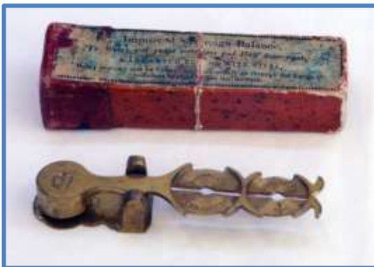
A brass sovereign and half-sovereign balance and its cardboard case. The case is principally red and pulls apart in the middle.
