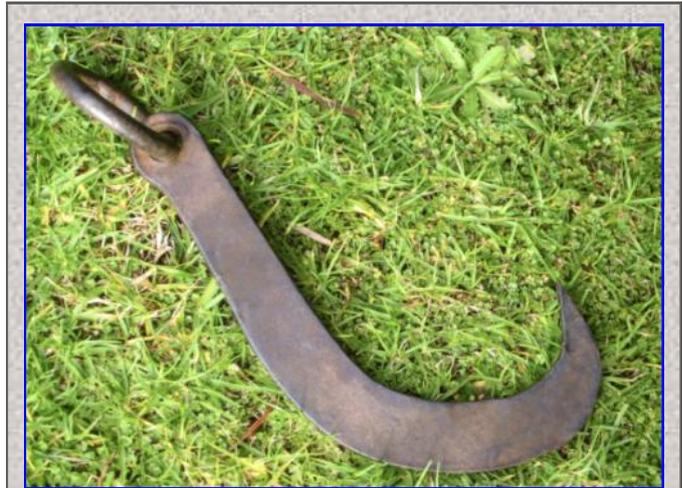
**ABOVE:** This is Laurie's cant hook. Sleeper cutters had several tools of trade, the cant hook being one of them. This hook was used to move logs and heavy timber using a bar through the ring for levering.
