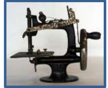
*A small hand-operated sewing machine. The body of the sewing machine is painted black. The top arm appears to have been painted in a white/cream colour. The machine could have been used to make small articles. There is no bobbin.*
