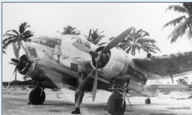
**ABOVE:** Beaufort A9-510/DD-S Bomber, similar to the plane which went missing on a training flight from East Sale. The Beaufort A9 was a twin-engine general reconnaissance aircraft powered by two Bristol Taurus 14 cylinder sleeve valve radial engines. Its maximum speed was 271.5mph, and range of 1,600 miles. It could carry bombs, mines, torpedoes, and was fitted with Vickers machine guns. Beauforts of this type were also converted into light transport planes.
