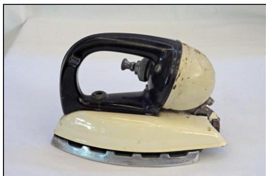
*This fuel iron (above) has a small cream-porcelain body and black handle. The back is a bulb-shaped container for holding the fuel. This is a kerosene operated Tilley Model DN 250n iron. It has a regulating generator which enables the user to control the heat.*
