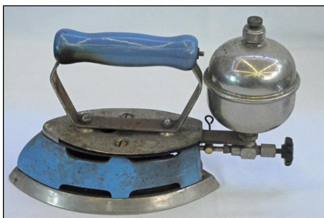
*This is a metal iron enamelled in blue colour, with a silver coloured fuel reservoir shaped like a bowl. This most likely stored Shellite which was the fuel to heat the iron. The handle is also blue and made of wood.*
