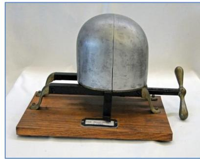
**Aluminium hat stretchers were generally in use from the 1920's. The hat was placed on the aluminium dome shaped piece; when the handle was turned, the dome section split vertically, one section moving away from the fixed half. A graduated scale along the side indicated the size.**
